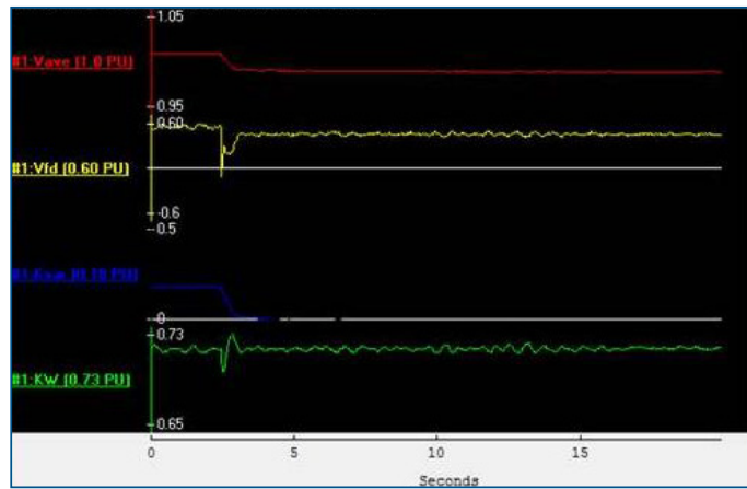
Figure 7b - A properly tuned PSS exhibits immediate damping after a small signal disturbance
